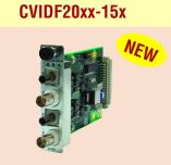
Transition Networks's Point System™ Chassis Video Media Receiver, when paired with our camera-mounted transmitter J/VD-TX-01, enables the transport of analog CCTV video over fiber infrastructure for extended reach video surveillance or security installations. And with Transition's unique Extended Fiber Receive Mode, the RX sensitivity can be adjusted to accommodate even greater fiber link distances.
