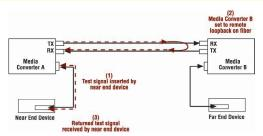
Some converters have separate copper and fiber loopback functions that can be enabled separately, while others will loopback both copper and fiber at the same time when enabled. Please refer to the specific product page for details.
