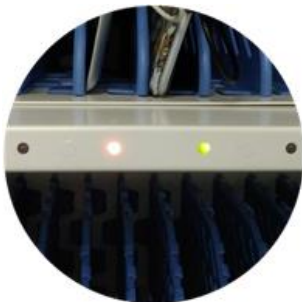
LED indicator designed in front of the slot which facilitate the power status monitoring
