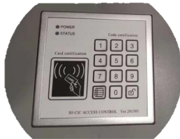
RFID & Keypad electronic lock, can be integrated to existing RFID cards
