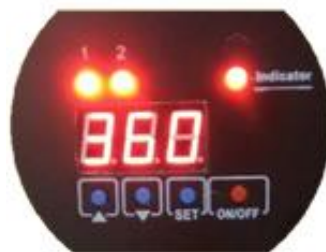
Timer design for power shut down automatically which facilitate the user to go out without monitoring
